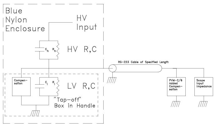
The probe is designed to produce the calibrated level of output with a 1 Megohm input impedance and with the specified cable length in place. Changes in cable length tend to change the calibration approximately 0.7 %/ft. for a typical 1000:1 probe. PVM-5 probes tend to have greater variations, while some PVM-1s have smaller variations. The 10,000:1 probes, including the VD series probes, have much smaller variations in calibration with cable length.
