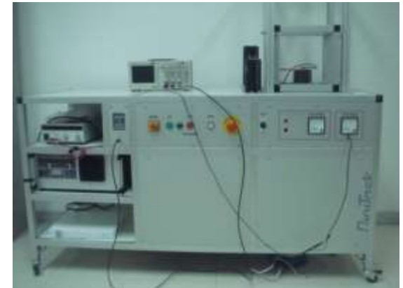
Transient Voltage Test
