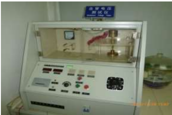
The Breakdown Voltage of Electrolytic Paper Pressure Tester
