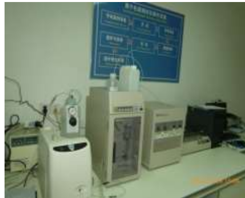
Quantitative detection of Chloride ion content of ion chromatograph
