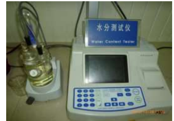
Detection and liquid electrolyte material of trace moisture tester
