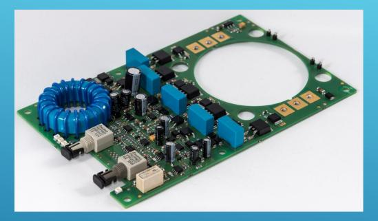
The high di/dt stacks are designed to switch high currents in a range of several 10'000Amps in a range of a few micro seconds. This applications are designed for high reliability and long endurance even under harsh environments. Typical applications are Thyratron replacements in radar systems where high availability over the years is mandatory.
